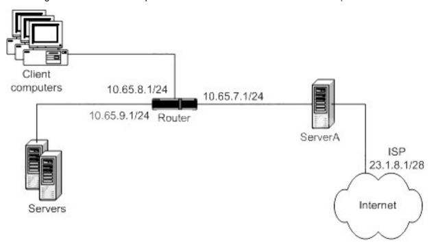
You want to configure the TCP/IP settings of the appropriate network adapter on ServerA so that client computers can connect to the Internet after you install ISA Server. What should you do?
