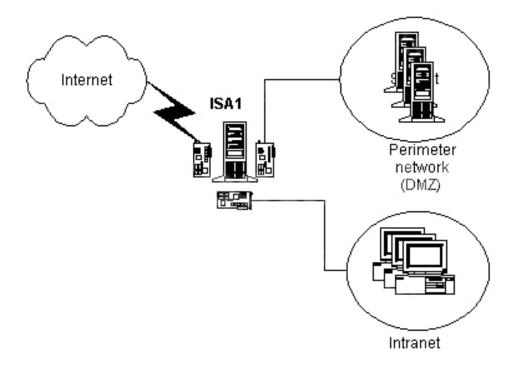
You also plan to add a Web server and an FTP server to the perimeter network (also known as the DMZ). Users on the Internet should be able to access the servers in the DMZ by using FTP and HTTP. Client computers on the company intranet should be able to connect to file shares on the servers in the DMZ. You need to configure ISA1 to support this functionality. Which two actions should you take? (Each correct answer presents part of the solution. Choose two.)
