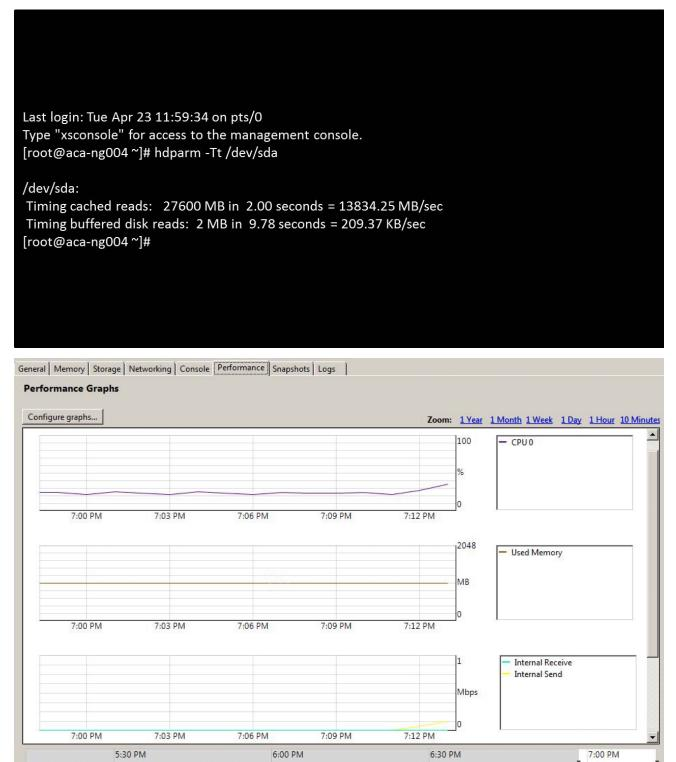
Which component, based on the attached exhibit, could be impacting performance?
