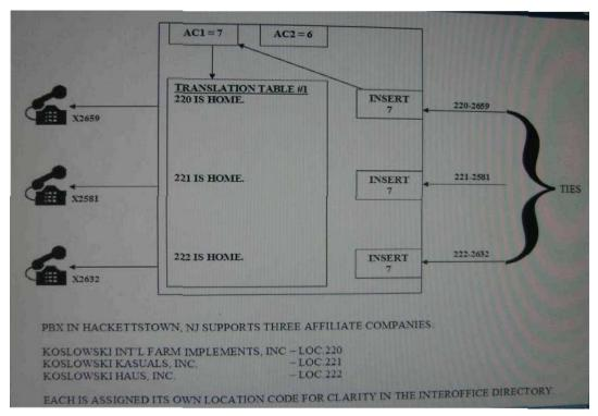
Consider a company so didi ng pi an sho wni nt he exhi bit and an example of crits require ments. A station user at the company, with Location Code 221, placed an ESN call, dialing 7-221-2581. This would be an On-Net call and the NARS programming must remove the LOC code and dial the DN internally.
