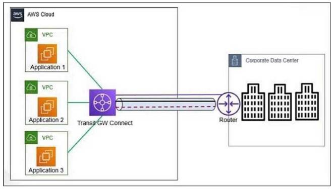
An organization deployed the application servers in the AWS VPC that connects to the corporate data center using Transit Gateway Connect. Demand for the applications has grown and the connection requires more bandwidth.
