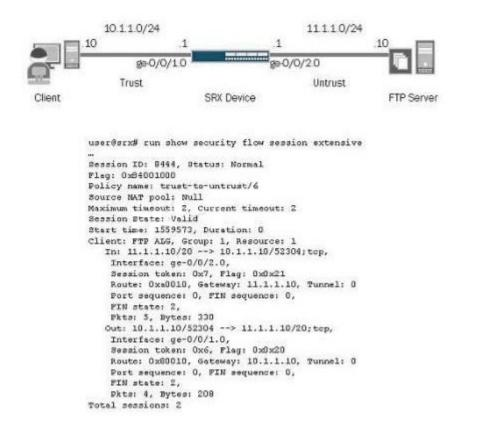
The client is downloading a file from the FTP server. The FTP control channel is established using a security policy named t rust-to-untrust.
