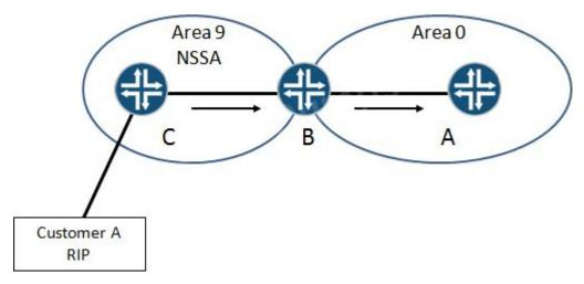
Referring to the exhibit, which type of LSA will be seen on router A for routes originating in Customer A's network?
