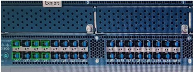
An administrator is building a FlexPod configuration with UCS 6296 Fabric Interconnect devices that support legacy Fibre Channel 9FC) connections. The administrator uses UCS Manager to configure the unified ports on the Fabric Interconnect.
