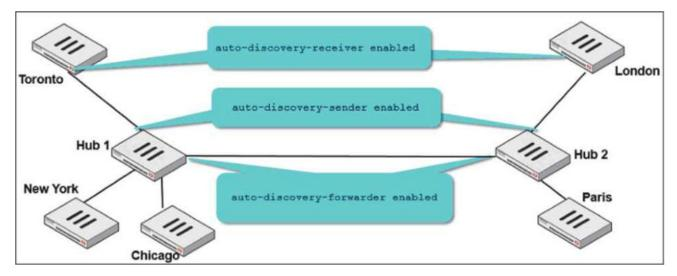
Two hub-and-spoke groups are connected through a site-to-site IPsec VPN between Hub 1 and Hub 2. The administrator configured ADVPN on both hub-and-spoke groups.
