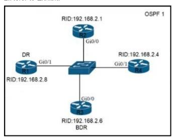
All routers in the network are configured R2 must be the DR. After the engineer connected the devices, R1 was elected as the DR.
