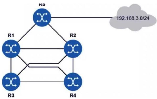
All routers in the diagram are running an interior gateway protocol (IGP) and have been configured with an ECMP value of 4. Router R5 advertises the prefix 192.168.3.0/24 using the IGP.
