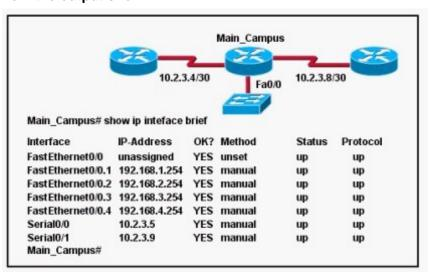
A.The LAN interfaces are configured on different subnets.
