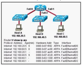
A.Router1 will strip off the source MAC address and replace it with the MAC address on the forwarding FastEthernet interface.
