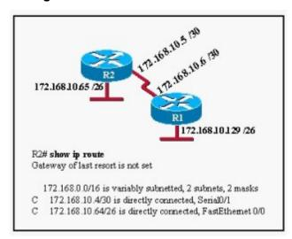
A.The serial interface does not have the clockrate set.
