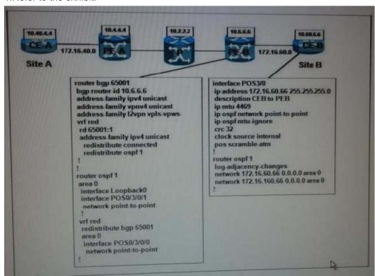
The customer has an MPLS Layer 3 VPN service CE-A is not able to ping the CE-B loopback address 10.60.6.6 CE-A is able to ping the CE-B network interface address 172.16.60.66. What must be added to the configuration to allow the loopback ping to work?
