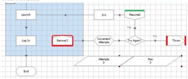
The Process is intended to attempt to perform the processing in the recover block, Block 3. a maximum of three times before throwing an exception.
