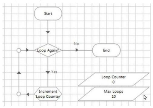
The data item "Loop Counter" is a number data item and has an initial value of 0. The data item "Max Loops" is a number data item and has an initial value of 10.
