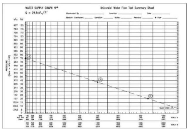
What is the residual pressure according to the water supply graph?
