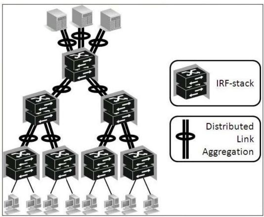
When IRF with Distributed Link Aggregation is implemented at all layers of a LAN (Core, Aggregation, and Access), which protocols can be replaced by IRF functions? (Select two.)
